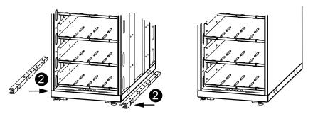
**NOTE:** The U-shaped anchoring brackets are 1-2 mm higher than the opening below the cabinet to disengage the casters. Therefore, the cabinet must be tilted when placing the U-shaped anchoring brackets under the cabinet.
