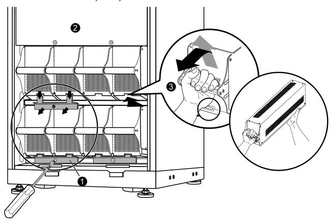
1. Remove all battery securing brackets (used to secure the batteries during transport) by removing the M6 Torx screws.
