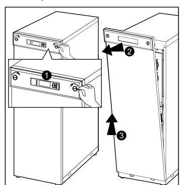
3. Lift the front panel free of the two slots at the bottom of the cabinet.
