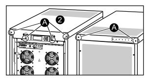
3. Remove the conduit plate at the back of the UPS top plate and drill holes centered in the small predrilled holes. 20 mm (3/4 in) is recommended for conduits.
