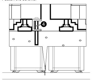
5. Move the adjacent cabinet on its casters close to the cabinet with the U-shaped floor anchoring brackets.
