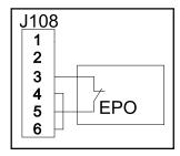
+24 V Normally Closed: EPO is activated when a SELV 24 VDC voltage is removed from pin 3 with reference to pin 4.
