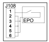
+24 V Normally Open: EPO is activated when an isolated SELV 24 VDC voltage is supplied on pin 1 with reference to pin 2. Connections: 3-5 and 4-6.
