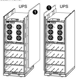
**NOTE:** Make sure that the cabinets are level so that they can be anchored to each other.
