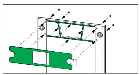
25. Remove the top gasket from the front panel.
