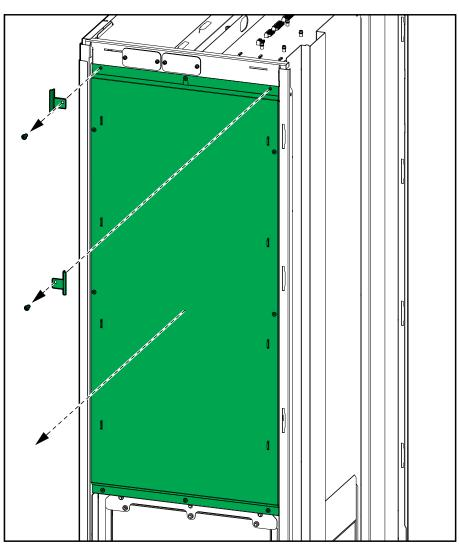
IP52 Kit for UPS Install the IP52 Kit on the UPS
