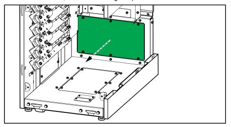
7. Mount the flat gasket 12.7 mm from the edges on the rear gland plate for optimal sealing and save the rear gland plate for later installation.
