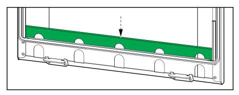
28. Install the four provided cage nuts.
