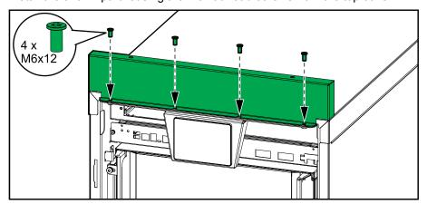
20. Install the shown part with the four provided M6 flat head screws and nylon washers.
