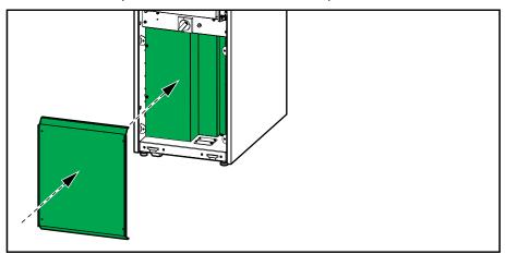
22. Remove the air filter from the front panel. Discard the air filter.
