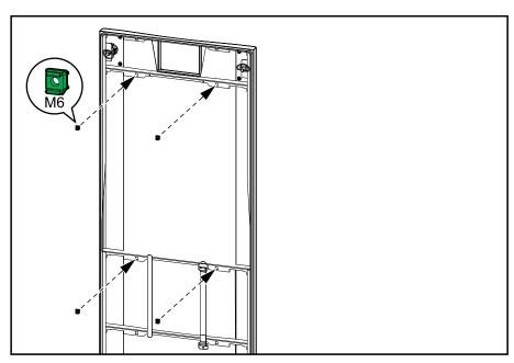
29. Install the shown part with the four provided M6 screws.
