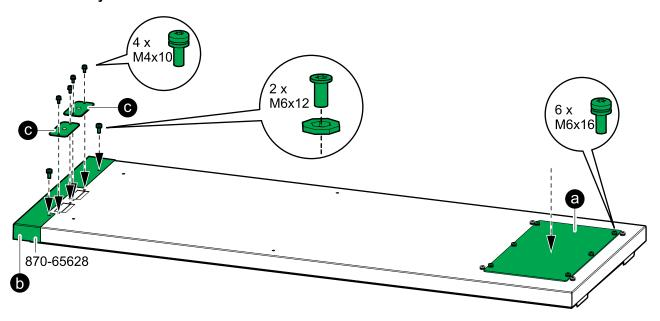
IP52 Kit for UPS Install the IP52 Kit on the UPS
