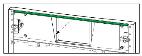
26. Mount the provided profile gasket as shown on the front panel as close to the edges of the front panel frame as possible. Start from the bottom centre and mount the profile gasket in one piece for optimal sealing.
