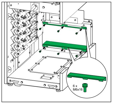
9. From inside the UPS, install the two shown parts on the bottom gland plate with the existing screws.
