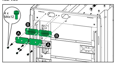
12. Reinstall the two brush plates reusing the four screws. Save the gland plates for later installation.
