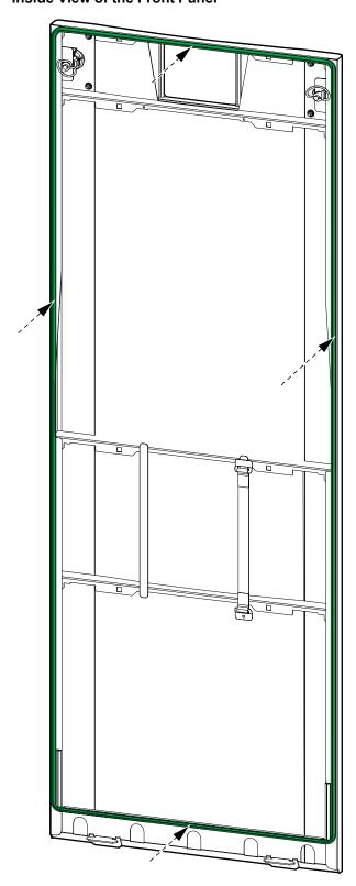
27. Install the transparent plastic part in the bottom of the front panel.
