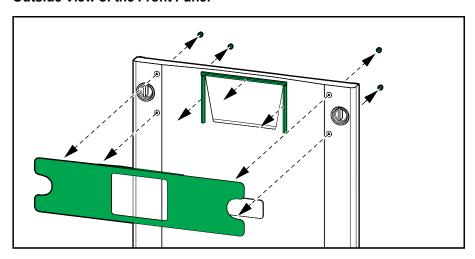
24. Mount the provided profile gaskets as shown and reinstall the display plate on the front cover.
