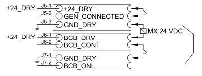
a. Connect the Aux switch signal cables from the empty battery cabinet to J6-2 and J7-1 in the UPS.
