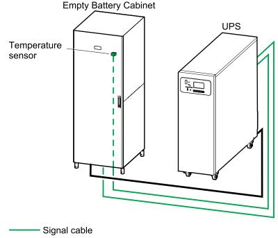
**NOTE:** The distance between the battery bank and the UPS must not exceed 200 m. Contact Schneider Electric for installations with a longer distance.
